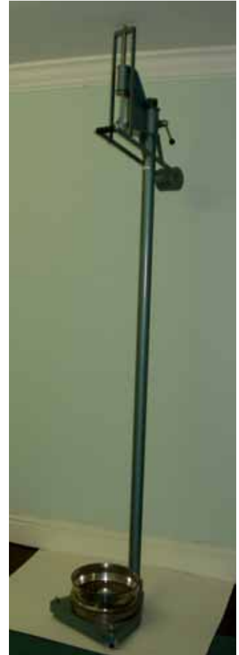
In accordance with the JCST specification the specimen falls exactly six feet (1.83 metres).
