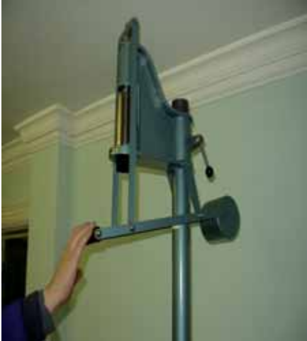
This method of ejecting the test Specimen ensures reproducible results.
