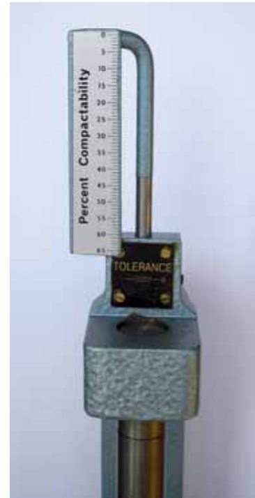
Compactability Scale Accessory mounted on Sand Rammer.
