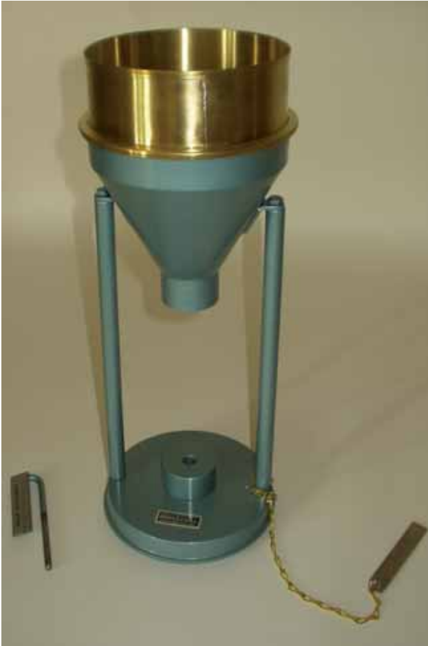
Filler Accessory for the consistent filling of the specimen tube.
